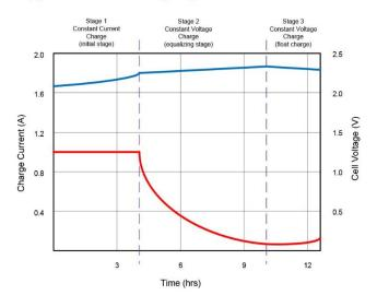
Typical *Cell charging* characteristics of the charger is shown in the table. The *Cell* is part of the battery, 12V batteries contain 6 cells and 24V batteries contain 12 cells.
