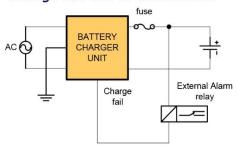
If reverse polarity protection is required, user has to fit an external fuse in the charge circuit with the indicated rating in the table.
