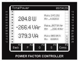
This screen displays total active, total reactive and total apparent powers, and minimum and maximum values of these powers.
