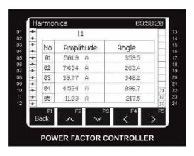
In the harmonics screen, each press on the table key will display the amplitude and angle of harmonic in tables.
