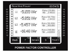
This screen displays reactive powers in phases, minimum and maximum values of these values, total reactive power, and minimum and maximum value of this value. If you press "Talep" (Demand) on this screen, the reactive power demand table will be displayed.
