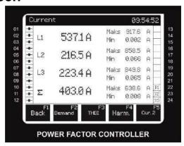
This screen displays the current values measured instantaneously for each Phase, and Maximum and Minimum current values.
