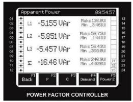
This screen displays apparent powers in phases, minimum and maximum values of these values, total apparent power, and minimum and maximum value of this value. If you press "Talep" (Demand) on this screen, the apparent power demand table will be displayed.
